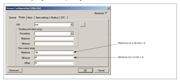
**Note:** In the **Trending and alarm range** section, the **Maximum** and **Minimum** values must be within the limits of the **Raw output range**.
